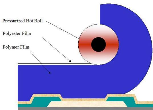
The main objective of the lamination step is to provide intimate contact between the polymer and the substrate, eliminating any air entrapment, ensuring the polymer flows into the substrate cavities encountered on the surface roughness, maximizing the polymer adhesion.
