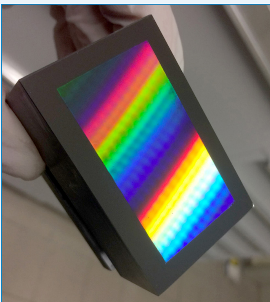
Diffractive optic: laminar grating (50 x 30 mm) 170 nm thick mr-P 1202LIL, 400 lines/ mm
