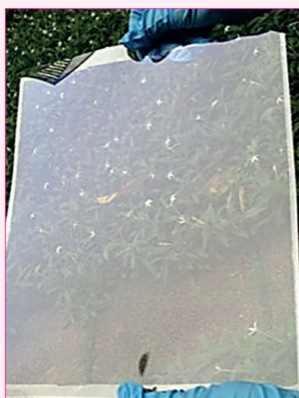
Antireflective coating on PC with mr-UVCur26SF: moth-eye pattern imprinted on PC foil in a R2R-NIL process (Courtesy of IMRE, Singapore)
