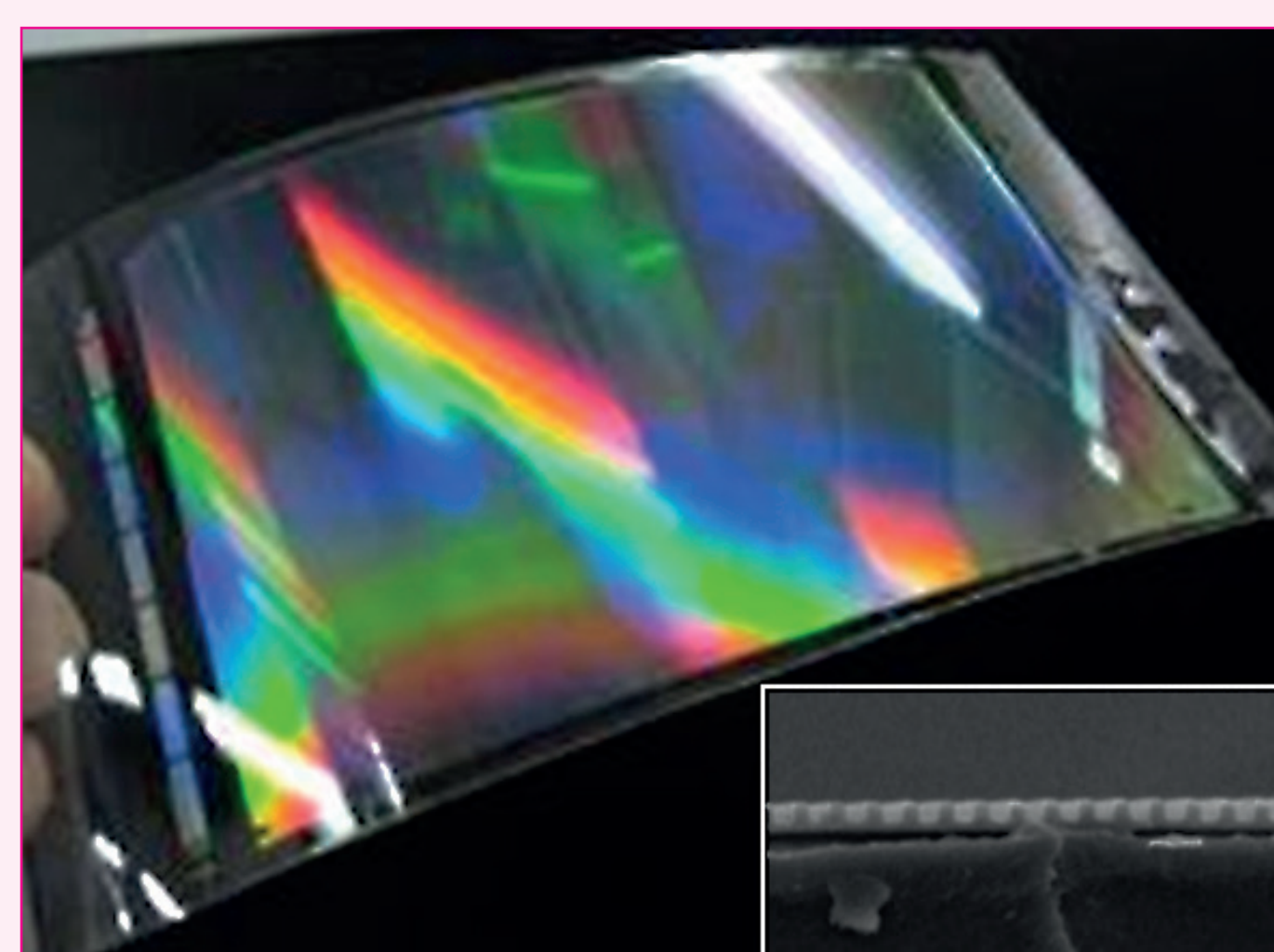
R2R-NIL on PC foil: AR1 L&S pattern, 500 nm pitch, inkjet dispensed mr-UVCur26SF, pristine Ni roller molds, 405 nm LED radiation, throughput speed 10 m min -1 (machine limit). Inset: SEM image of the imprint (Courtesy of IMRE, Singapore).
