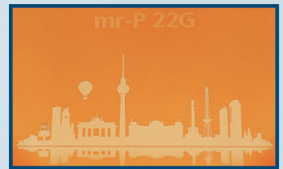
Greyscale pattern in mr-P 22G by DWL @ \lambda = 405 \text{ nm} with DWL 66+ 1)
