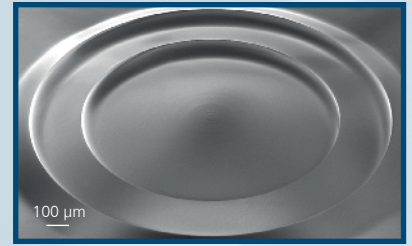
103 \mu\text{m} high, 2 mm diameter Fresnel lens 1) (DWL66+)
