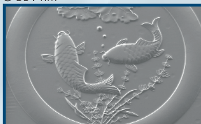
Test pattern, 63 µm pattern depth, patterned by Heidelberg Instruments
