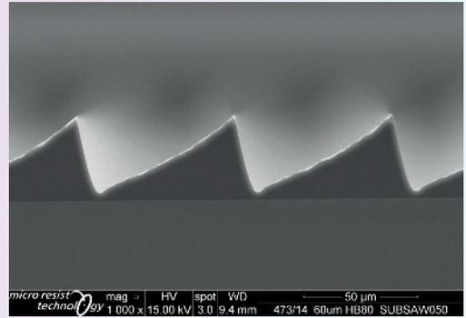
Aperiodic saw tooth pattern in ma-P1200G with pattern depth approx. 40 µm using greyscale chromium mask photolithography process
