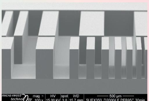
Test pattern made of SUEX dry film with 350 µm film thickness exposed with i-line filter
