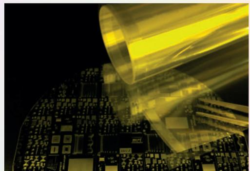
In-house fabricated roll of mr-LamiRes dry film resist with 50 µm layer thickness, laminated on a 100 mm wafer and patterned by UV mask-aligner
