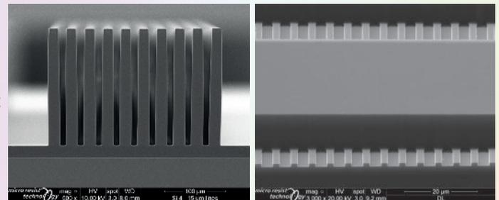
SU-8 lines and spaces with 180 μm height on top of 20 μm SU-8 base layer made by UV-lithography
