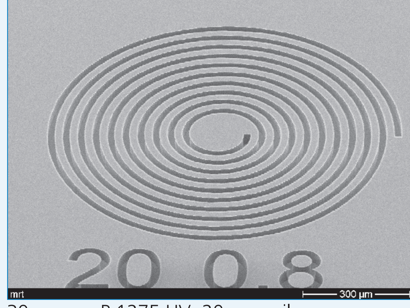
30 µm ma-P 1275 HV, 20 µm coil
