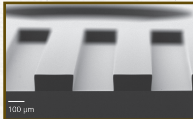
Binary test pattern for UV lithography in OrmoComp®
