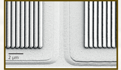
Slanted gratings in OrmoStamp® fabricated by replication (Courtesy of NILT, Denmark)
