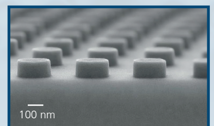
Patterned SiN using selective material deposition via inkjet and subsequent NIL+etch (Courtesy of Fraunhofer ENAS, Germany)
