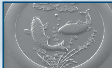
63 µm deep pattern in ma-P 1275G, patterned by Heidelberg Instruments
