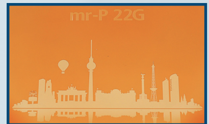
Greyscale pattern by DWL @ \lambda = 405 \text{ nm} (DWL 66+) 1)
