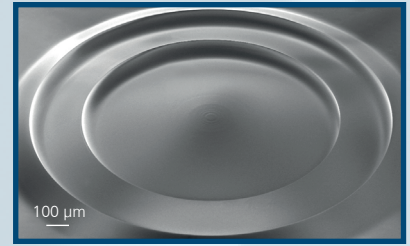
103 \mu\text{m} high, 2 mm diameter Fresnel lens 1) (DWL66+)
